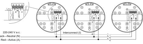
Max Interconnected Alarms: 40 Max. wiring length between first and last alarm: 150 m
